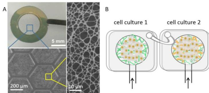
**Figure 1.** (A) Photograph and SEM images of a culture patch after electrospinning. (B) Scheme of the 2-chamber microsystem to be developed.
